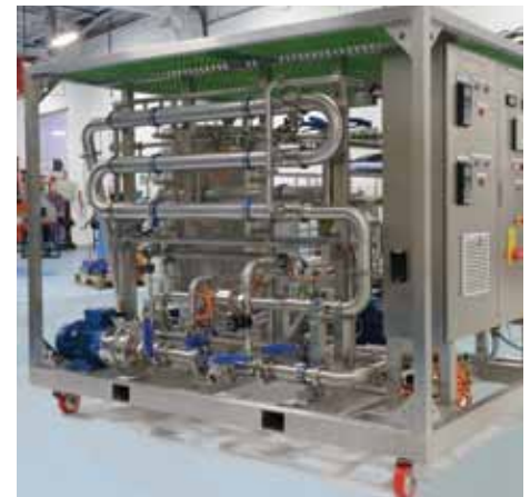
Microfiltration / Ultrafiltration pilot plant
