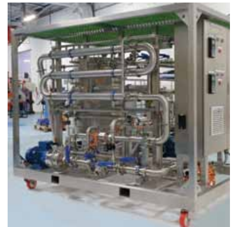
Microfiltration / Ultrafiltration pilot plant
