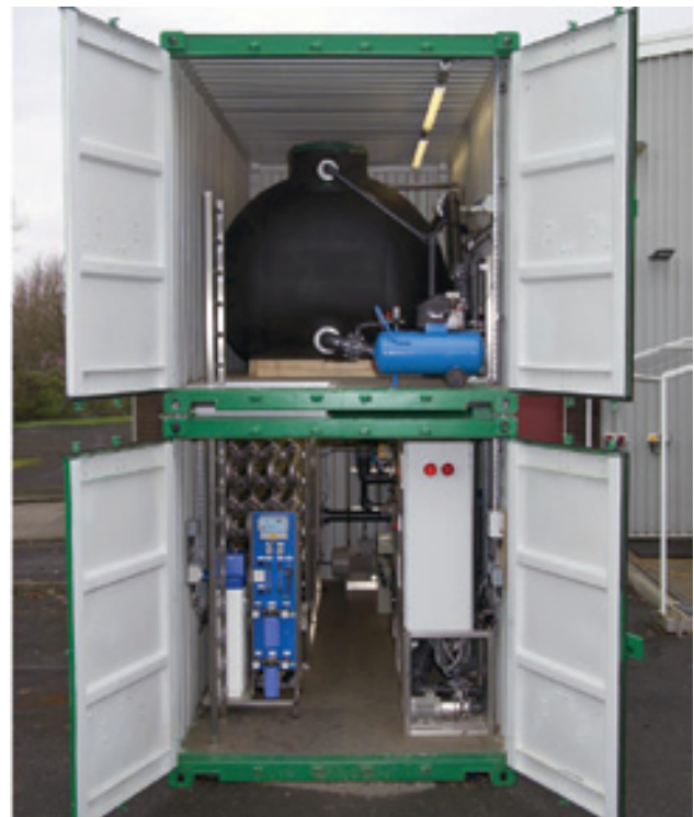
Containerised systems provide flexibility of location, easy transportation and low-cost installation
