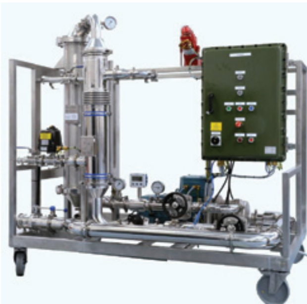
Mobile ATEX ZONE 1 rated membrane filtration system for pharmaceutical application
