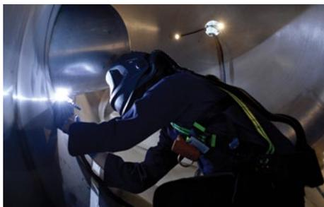
Available welding processes include Orbital or Manual TIG Welding, conforming to ASME IX and BS EN ISO 15614-1:2017 Standards.
