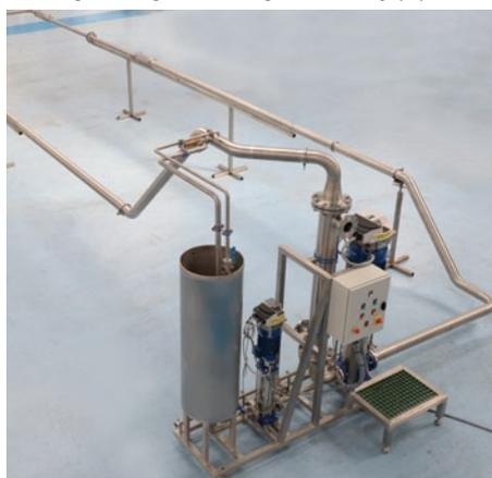
As part of the testing process Rototherm commissioned Axium Process to help design and build a 316 stainless steel vibration test skid. Adjustments of upstream pressures are made by varying sized orifice plates with test pressures of up to 16 Bar.
