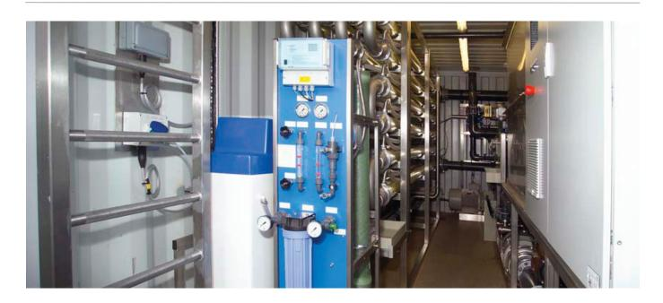
Axium Process specialises in crossflow membrane technology and is working with companies wishing to evaluate the benefits of membrane filtration as a treatment for wastewater and separation of microplastics. Our expertise is in the design, build and commissioning of customised membrane filtration systems that provide a simple, compact and efficient solution for separating out contaminants and recovering clean, reusable water without the addition of chemicals.
